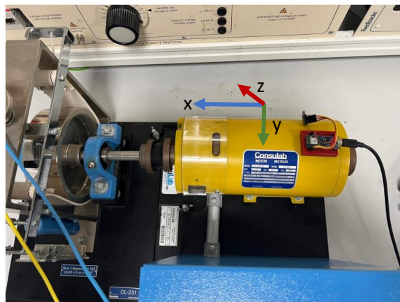
Figure 1. The experimental setup showing the DC electric Motor coupled to the load and the Arduino board on the top end of the motor
